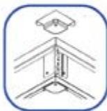
Securing top and bottom corner brackets
